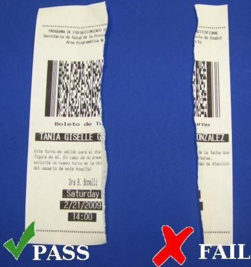
Figure 6. Vertical Test. The next ticket was torn vertically. The larger half successfully scanned while the narrow half did not.
