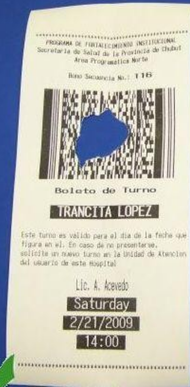
Figure 7. Central Removal Test. A large section was removed from a ticket. The remaining piece still scanned, while the removed piece did not.
